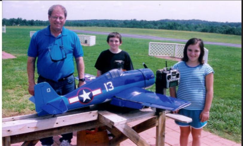
Ron's uses a Futaba radio in the F6, a Hangar 9 ARF. Ron added segmented flaps to the War Bird and installed Robart rotating retracts. His 4 stroke Saito 115 provides plenty of power and allows Ron to show what it can do.
